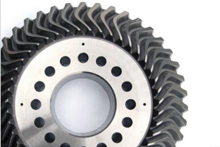
Bierens was the first who used 5 axis milling machines for the production of gears, in particular required for spiral bevel gears. Dr. ir. Noud van Roosmalen (Head Technical Department): "The software was developed in house and successfully applied. The development and expansion of this software is the core task of the Bierens' department of Technology & Development."
